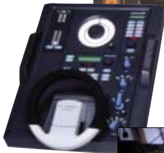
Autopilot Control Stand Upper Panel
